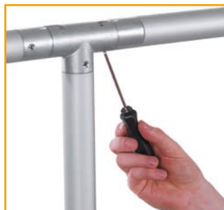
Loosen clamping screw
