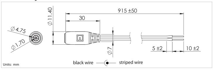
**tolerance** X: ±0.5 mm .X: ±0.3 mm .XX: ±0.05 mm applicable unless otherwise indicated in specification or on drawings Tensility International Corporation reserves the right to substitute parts which are functionally equivalent to the ones specified.
