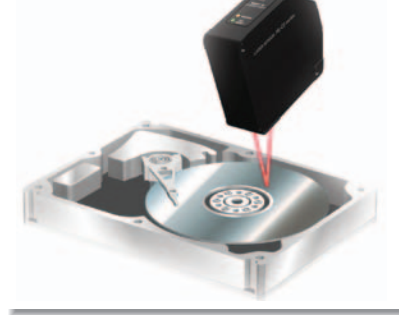
Measurement of HDD surface variations
