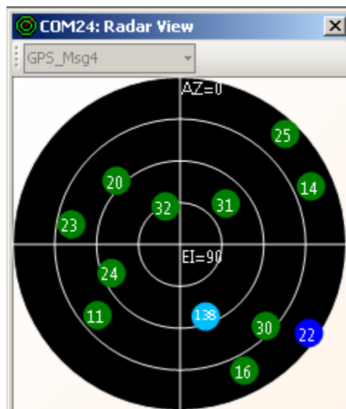
Figure 10: Displays the satellites by azimuth and elevation.
