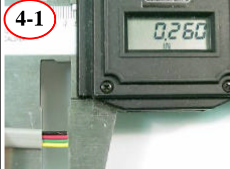
Remove @ 0.260" of cable jacket
