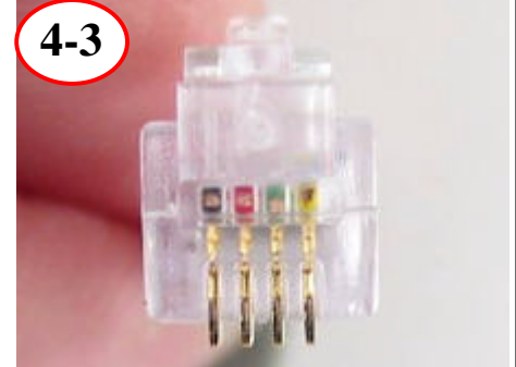
Verify wires went to end of plug housing, then crimp
