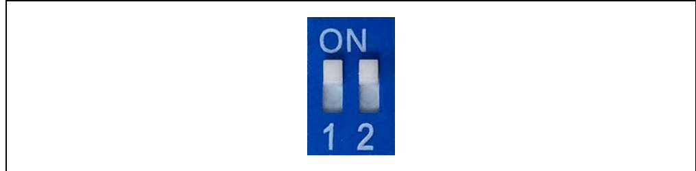
FIGURE 3-36: SWITCH SW9 IN ROM TEST MODE
