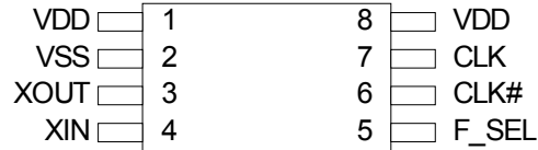
Figure 1. Pin Diagram - 8 Pin TSSOP
