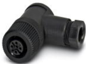
Connector, 5-position, Socket angled M12, A-coded, Screw connection, knurl material: Plastic, cable gland Pg7, external cable diameter 4 mm ... 6 mm
