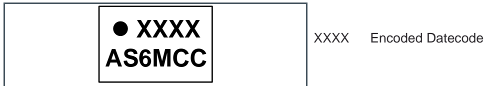
Figure 37: WLCSP Package Marking/Code
