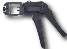
436 52 Crimping Tool Frame Parallel action ratchet crimp tool designed to provide the best crimp without compromise on modular plug terminals. Ratchet action to ensure full crimp cycle with safety release.
