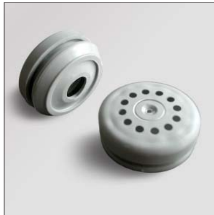
Vent plugs with labyrinth seal to prevent the formation of condensation; IP x 4; for wall thicknesses of 1.5 - 4.5 mm
