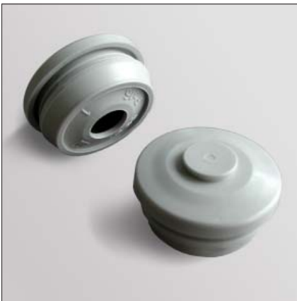
Double membrane cable glands IP 66, with 2 integrated sealing membranes, interference fit without counter-nut, for wall thicknesses of 1.5 - 4.5 mm
