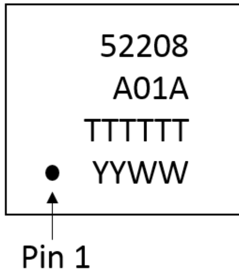
Figure 10.10. Si52208 Top Marking
