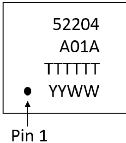
Figure 10.11. Si52204 Top Marking
