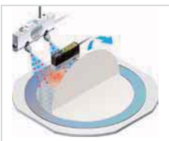
Measuring surface potential when removing BG sheets
