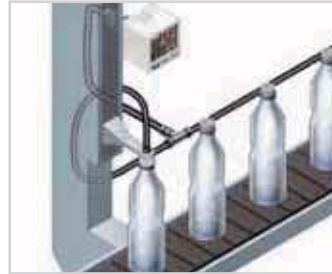
Air-leak test for PET bottles
