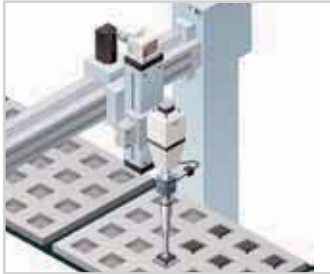
Confirming suction of electronic component
