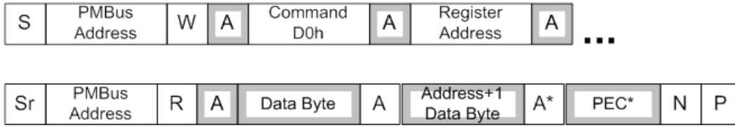
Figure 63: SMBus Custom Process Call to Read an internal Register
