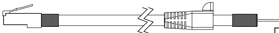
-S IN-PROCESS 3 TERMINATE FIRST END TO CONNECTOR (SAME AS -D IN-PROCESS 3, UNLESS OTHERWISE STATED)
