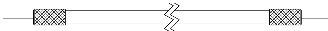
-BC IN-PROCESS 2 (FOLD SHIELD BACK OVER JACKET) (SAME AS -D IN-PROCESS 2, UNLESS OTHERWISE STATED)
