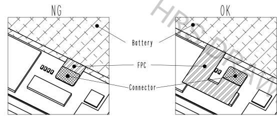
\*Possible problems caused by connector mating in incorrect positioning.
