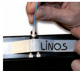
Pressing down and repositioning a mirror on the fixed mirror mount
