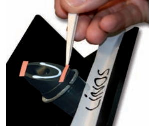
Positioning paper strips as spacers on a mirror mount
