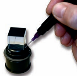
Applying adhesive in spots between optics and contact surface of the holder
