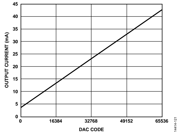
Figure 138. Gain Curve for ANA_FULL_SCALE_CURRENT[9:0] = 1023, DAC Offset = 3.8 mA
